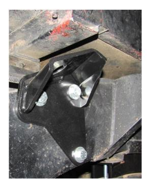
Fit new bracket to chassis using new M10 hardware supplied as shown.
